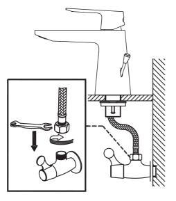
Connect flex water supply lines to angle stops and tighten with adjustable wrench. Turn on both hot and cold main valve Apply pipe tape (optional)
