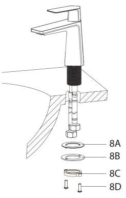
Install faucet through 1-3/8" predrilled hole in countertop. Attach rubber washer (8A), metal washer (8B), mounting nut (8C), and mounting screws (8D) on the threaded mounting pipe. Tighten mounting nut (8C) until snug. Tighten screws (8D) on mounting nut (8C) with Phillips head screwdriver until snug
