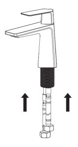
Place faucet on a soft cloth, spout facing up. Connect the waterlines to the base of the faucet (HAND-TIGHTEN ONLY) (A)Hot side left (B)Cold side right
