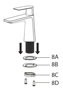
Remove the mounting screws (8D), mounting nut (8C), metal washer (8B), and rubber washer (8A) from the mounting pipe
